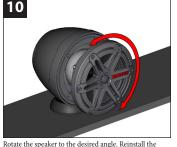
speaker and speaker to the desired angle. Reinstall the speaker and speaker mounting screws and washers. Hand-tighten in a criss-cross pattern.
