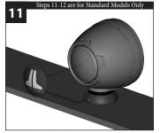
Remove the backing from the rear logo appliqué. With the logo positioned at the desired angle, attach the appliqué to the back of the enclosure.
