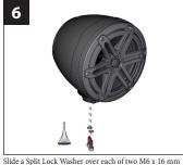
Slide a Split Lock Washer over each of two M6 x 16 mm Socket Cap Machine Screws, apply Loctite\* Red Thread Locking Compound, and fully tighten into the Fixture Base. Repeat for the third fastener. Continue to Step 8.
