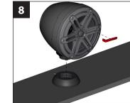
Align the keys of the Mounting Base with the keyways in the Mounting Receiver, then insert fully. Aim the speaker in the desired direction, and tighten the Set Screw in the Mounting Receiver. Remove adhesive backing and install the JL Audio logo badge.
