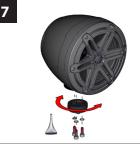
Remove the fasteners from Step 1, and rotate the Mounting Base to align with either the next or previous mounting hole in the Fixture Base. Slide a Split Lock Washer over each of three M6 x 16 mm Socket Cap Machine Screws, apply Loctite\* Red Thread Locking Compound to the screws, and fully tighten into the Fixture Base.
