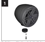
Hand tighten one M6 x 16 mm Socket Cap Machine Screw and Split Lock Washer to temporarily secure the Mounting Base to the Fixture Base of the enclosure, as illustrated.
