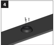
Mark the three mounting hole locations with a pencil, and drill pilot holes on the marks with an appropriate drill bit. Install the Mounting Receiver with three #10 x 1" Flat Head Phillips Sheet Metal Screws. Insert the Mounting Base into the Mounting Receiver, rotate the enclosure to the desired position, and tighten the Set Screw.
