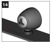
Align the aluminum logo cap to the desired angle of rotation, and press it onto the back of the enclosure. Apply masking tape (not included) to hold the cap in place until the silicone cures (at least 24 hours).
