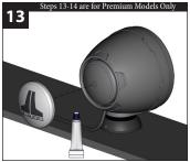
Clean the inside of the aluminum cap with acetone (not included) prior to attaching it to the enclosure. Apply a circular bead of silicone adhesive to the inside of the aluminum logo cap, 1/2-inch (13 mm) from the outer edge.
